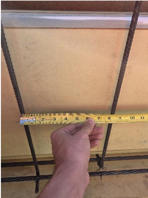
Figures 6: 8.25 in. Stirrup Spacing and 6.50 in. Stirrup Spacing
