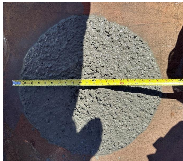
Figures 7: Spread Test Set Up and Spread Test Results
