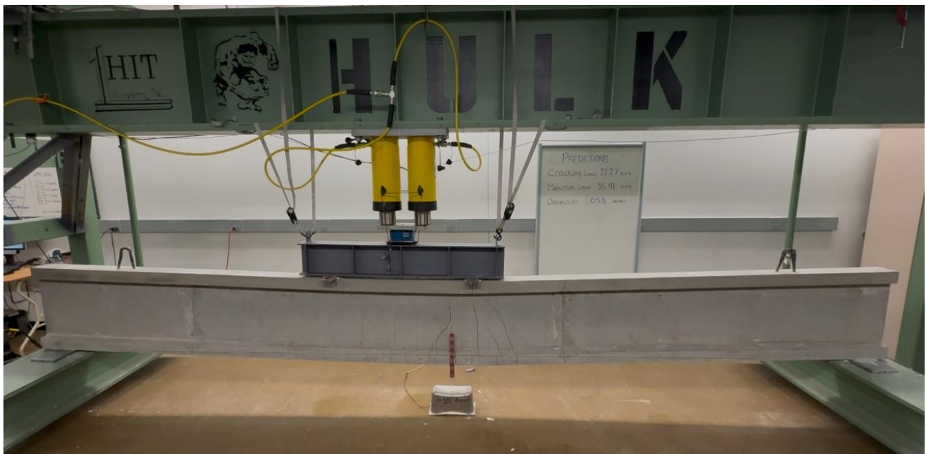
Figure 12: Cracking Under Load
