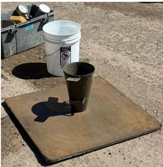
Figures 7: Spread Test Set Up and Spread Test Results
