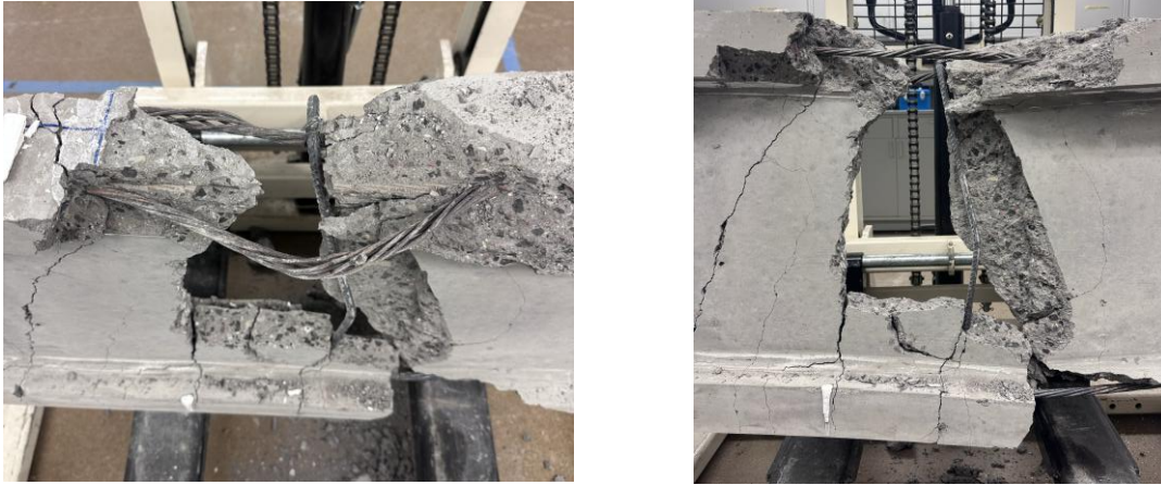
Figures 13: Beam at Failure Top View and Side View
