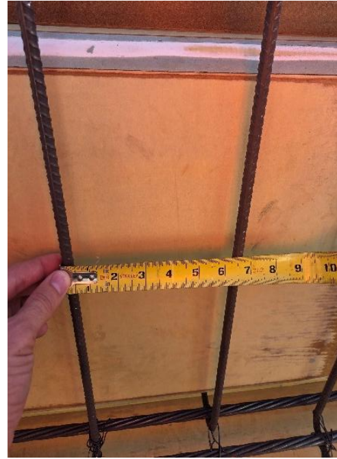
Figures 6: 8.25 in. Stirrup Spacing and 6.50 in. Stirrup Spacing
