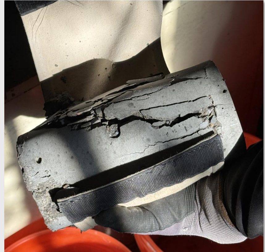
Figure 22: Broken Test Cylinder
